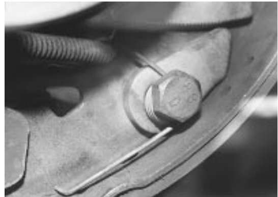
This bolt was substituted during a repair job.
