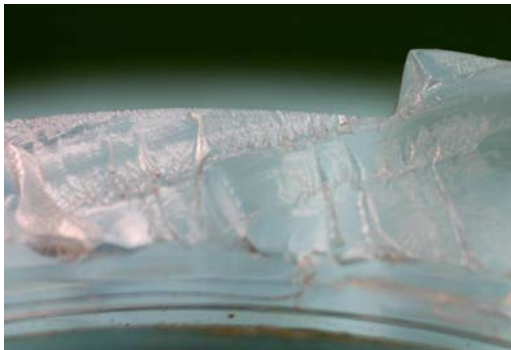
Microscopic view of water filter failure
